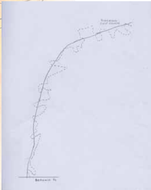
Original course of Dandenong Creek – dotted line; Re-alignment undertaken by Dandenong Valley Authority, 1967-71 – full line"
